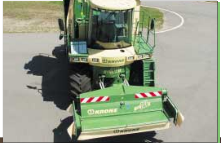
Compact through and through: Converts from 9.70 m mowing width to 3 m transport width without leaving the cab. The layout in transport ensures a high degree of safety and a clear view for driving on roads with heavy traffic.
