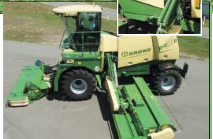
Optimum guidance: Spring relief packages reduce the contact pressure of the side mowers and provide the optimum contour following on the ground and are adjusted manually by means of a bolted central coupling bar. Hydraulic adjustment is available as an option.
