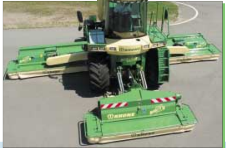
BiG M II, the mowing giant: 9.70 m mowing width with three EasyCut mower units and CV high-performance conditioners or 9.00 m with CRi conditioner rollers. The mower units all function independently with a clean cut always guaranteed.
