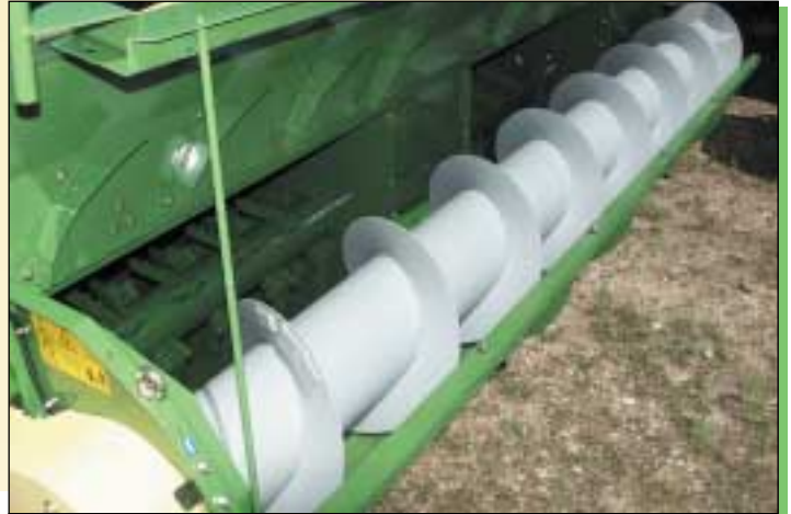
View of the guide plates: Guide plates are integrated in the hood for reliable conveyance of the crop to the centre.
