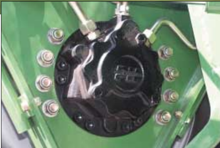
Hydraulic drive train: The drive train of the all-wheel drive BiG M II is unique on the market. Four radial piston motors help the machine to achieve what is impossible with conventional drive trains.
