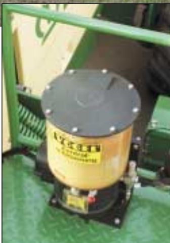
For reduced downtime: Optional central lubrication for all three mowers!
