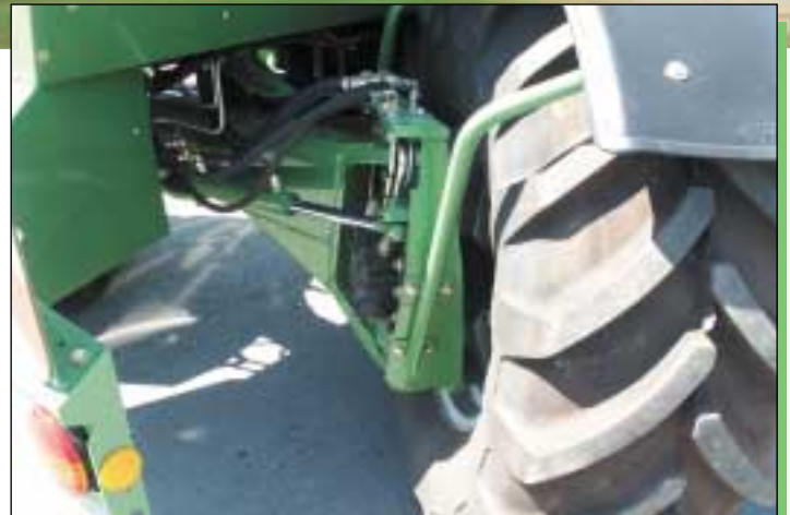
The view from above proves it: The rear axle steering and the hydraulic drive train make the BiG M II so manoeuvrable that maximum output is possible even in confined spaces. Therefore, the self-propelled mower conditioner from Spelle is viable even when used for cutting smaller fields.
