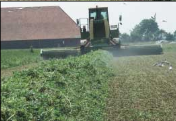
Closed: The view from the rear shows the compact unit, completely enclosed, that reliably channels the forage to a swath with a width of 1.80 m.
