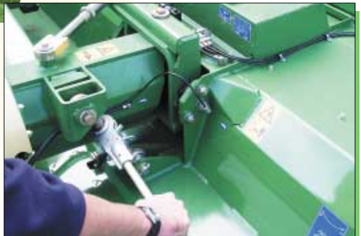
One movement of the hand: Adjustment of the cutting height on the side mowers is fast and easy. This allows you to quickly adapt the mowers to the local conditions.
