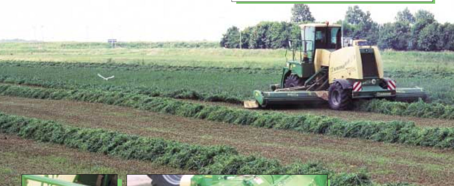
Clean: The BiG Swath System with a CRi conditioner in lucerne. Without touching the ground, the augers transfer the crop on to the swath produced by the front mower.
