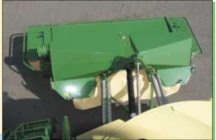
An excellent cut across the entire mowing width, even on slopes, with the optional front mower steering kit: The frame of the front mower can be moved to the left and right by means of a hydraulic cylinder adjusting the overlap to the side mowers.
