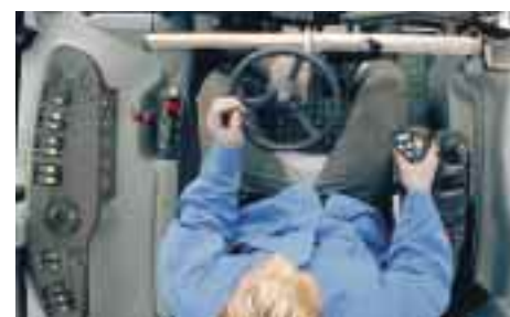
Reverse drive facility* adding even more versatility and productivity by simply rotating the driver's seat to face a second steering wheel.
